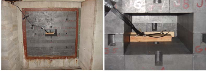
Figure 70. Diode mount placement in thermal column.
